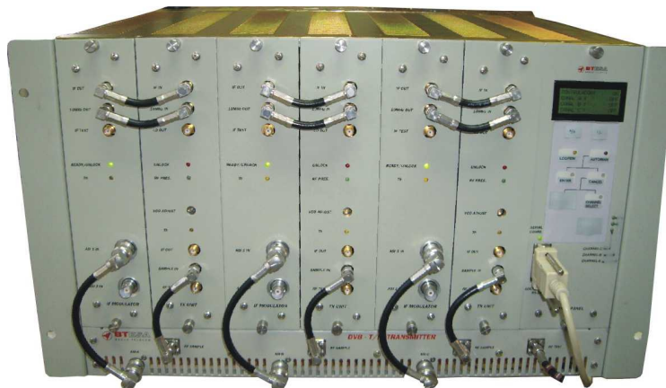
3 channel / 5Wrms DVB-T Gap-Filler
